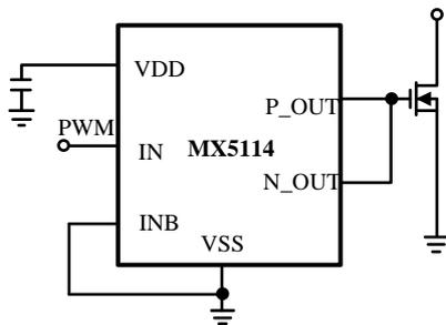
Figure 6 Noninverting Application
