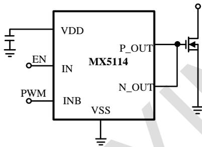
Figure 7 Inverting Application
