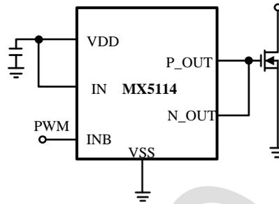
Figure 9 Inverting Application With Enable Pin
