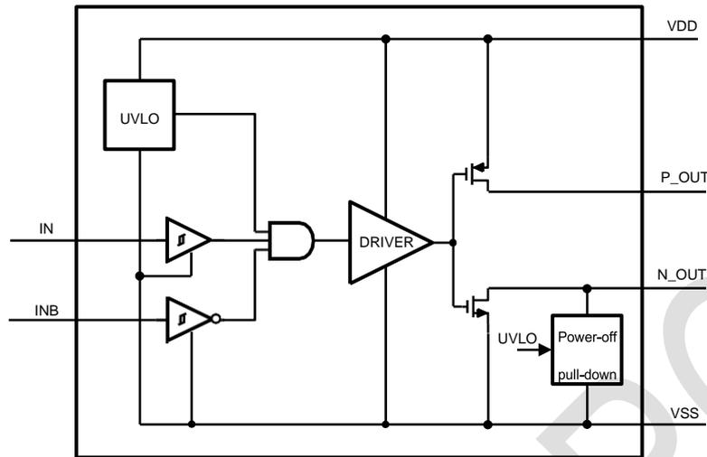
Figure 1 MX5114 Block Diagram
