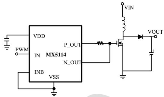
Figure 5 Simplified Boost Converter
